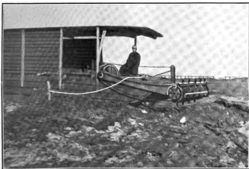
FIG. 1.—POWER-DRIVEN MACHINE FOR FREEING CHANNELS OF SEDGES AND SALT GRASSES, MISSEGUASH MARSH, NEW BRUNSWICK.
